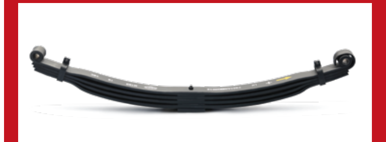
Front Parabolic Suspension for higher ride comfort
