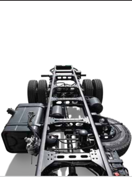
High Strength Low Alloy (HSLA) material chassis
